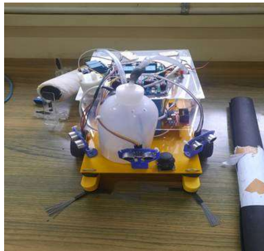
Fig 7.5.1: IoT Based Automatic and Manually Controlled Floor Cleaning Robot
